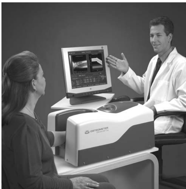
Fig. 15-20. The Osteometer DEXACare® G4. A peripheral dual-energy X-ray absorptiometer. Photograph courtesy of Osteometer MediTech, Hawthorne, CA.
